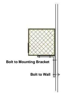
L-Brackets should be 6" from the ends of the unit
