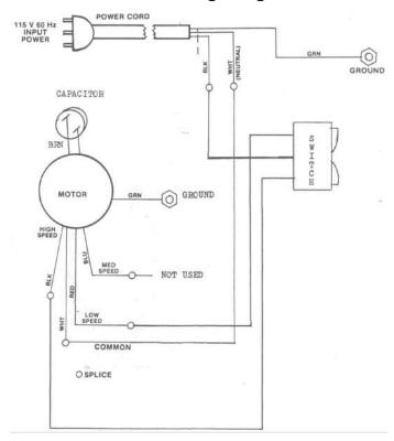
CL2500 w/ 3 Speed Switch Wiring Diagram
